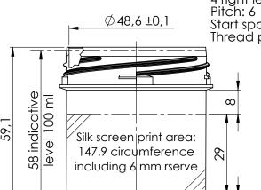
4 right leading threads Pitch: 6 Start spaced at 90° Thread pitch of 162°
